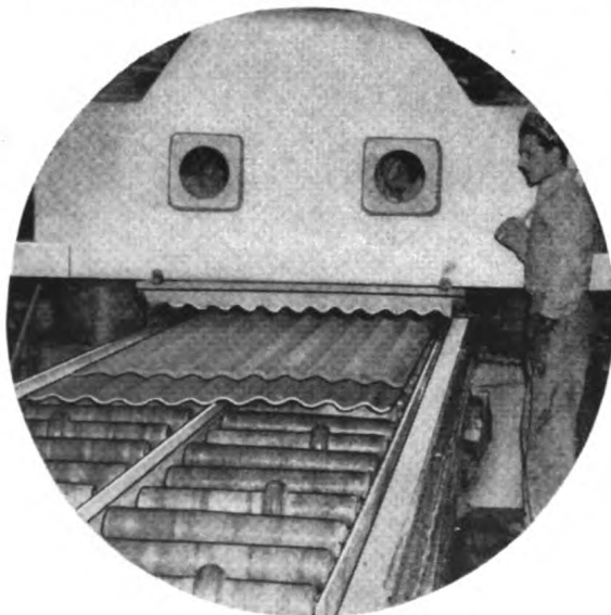
Hydraulic pressing of freshly formed corrugated asbestos-cement sheets.
